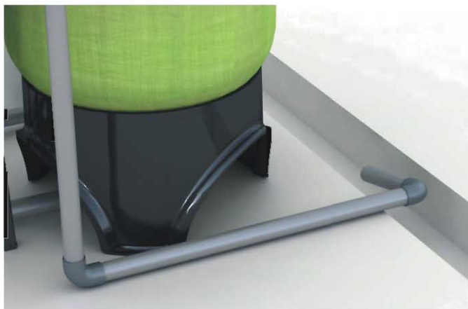
Figure 1-2 Correct Way of Drainage
