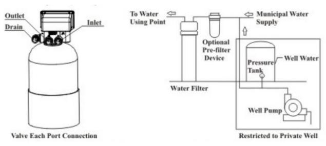
\*It is suggested to install a manual bypass valve between the main water inlet and inlet/outlet of the device, making it convenient for installation and maintenance. (Refer to the below installation picture).
