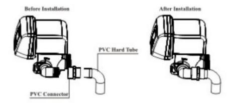
\*Control valve should be higher than sewer. The length of drain line should be similar to the height of tank. Insert the drain line to the floor drain, but not to the bottom. Leave about 5-10mm distance between the end port of drain line and sewer.
