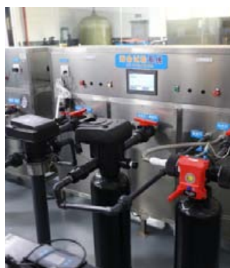
球阀寿命检测 Ball valve lifetime test
