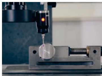
阀杆检测 Valve shaft inspection
