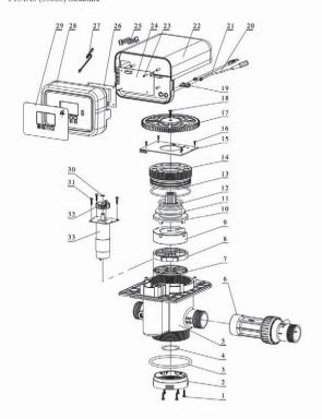
Component and part No. for F134A1/F134A3 (Components for F134A1without No.6 and No.21)
