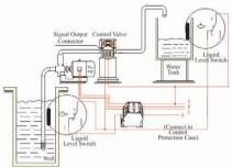
Figure 3-5 Wiring of Liquid Level controller controlling Inlet Pump
